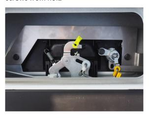
2) Remove the two screws that hold the tailgate handle into the tailgate, Also unclip the locking Rod
