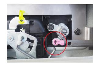
5) Attach the Power Lock to the vehicles lock barrel (use new rod lock clip provided) re insert the locking rod into new clip
