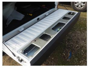
3) Install the base plate and actuator kit, hold in place by replacing the removed screws from no.2
